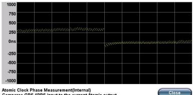
Atomic Clock Phase Measurement(Internal) Compares GPS 1PPS input to the current Atomic output.
